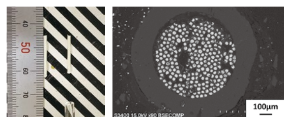
Fig. 3 Photograph of bundled OCS (left), 1 mm thick bundled OCS plate (right)
