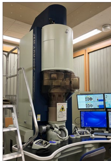
Fig.1 TEM equipped with aberration correctors both in illumination and objective lens systems. This microscope is open to users outside the campus.
