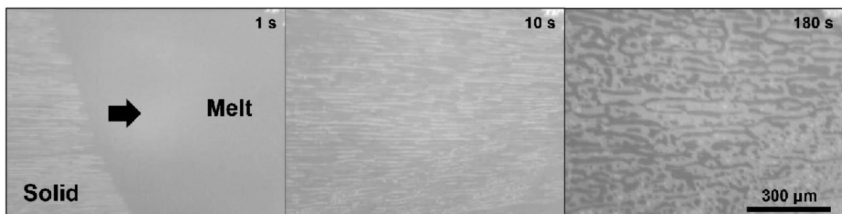
Fig. 1 Snapshots of solid/melt interface during directional solidification of Ni 44 Si 56 alloy and the subsequent microstructure evolution at a cooling rate of 2\text{ }^{\circ}\text{C min}^{-1} , recorded using an optical microscope at different times. The growth direction is toward the right [1].
